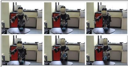
The iCub robot grasping an object on the table.
